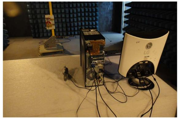
POWERLINE CONDUCTED EMISSIONS SETUP PHOTOS
