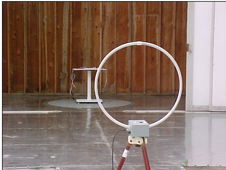
View of the EUT during Radiated Emission Testing on the 10 Meter OATS, measurement of Low Frequency Signals
