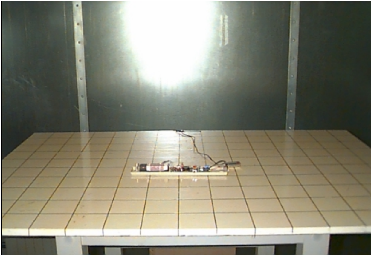
Front view of the Homecare during the Conducted Emissions tests in the Shielded ESD room.
