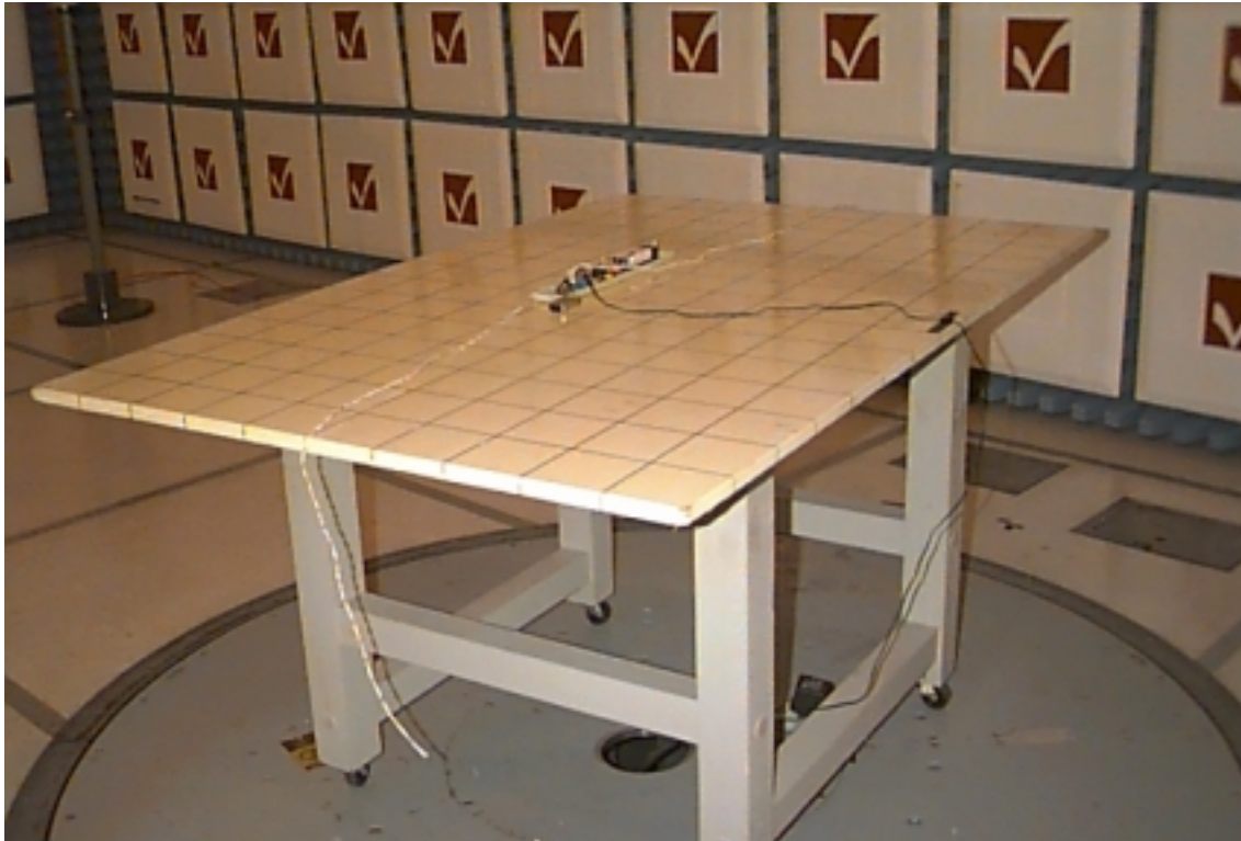
Rear view of the Homecare Alarm Unit during the Radiated Emissions tests in the 3-Meter FCC listed Semi-Anechoic Chamber
