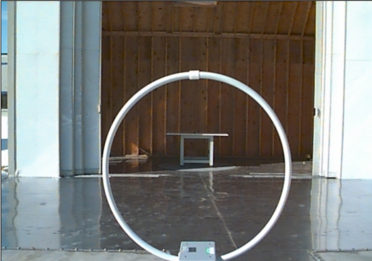
Front view of the Homecare Alarm Unit during the Radiated Emissions tests using the Loop Antenna on the 10-Meter FCC listed OATS
