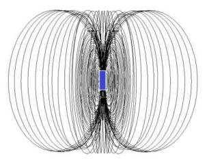
The TX antenna coil is what's called an "autotransformer", which is a transformer where the primary and secondary are one piece of wire (18 gauge) common to a tap point wrapped around a ferrite core (4.875" x 0.125" x 0.25". The "turns ratio" makes it a step-up transformer; and the tap point is optimized for a tradeoff between "transforming up" to the highest possible voltage, and also impedance matching the antenna to the driver for maximum power transfer.
