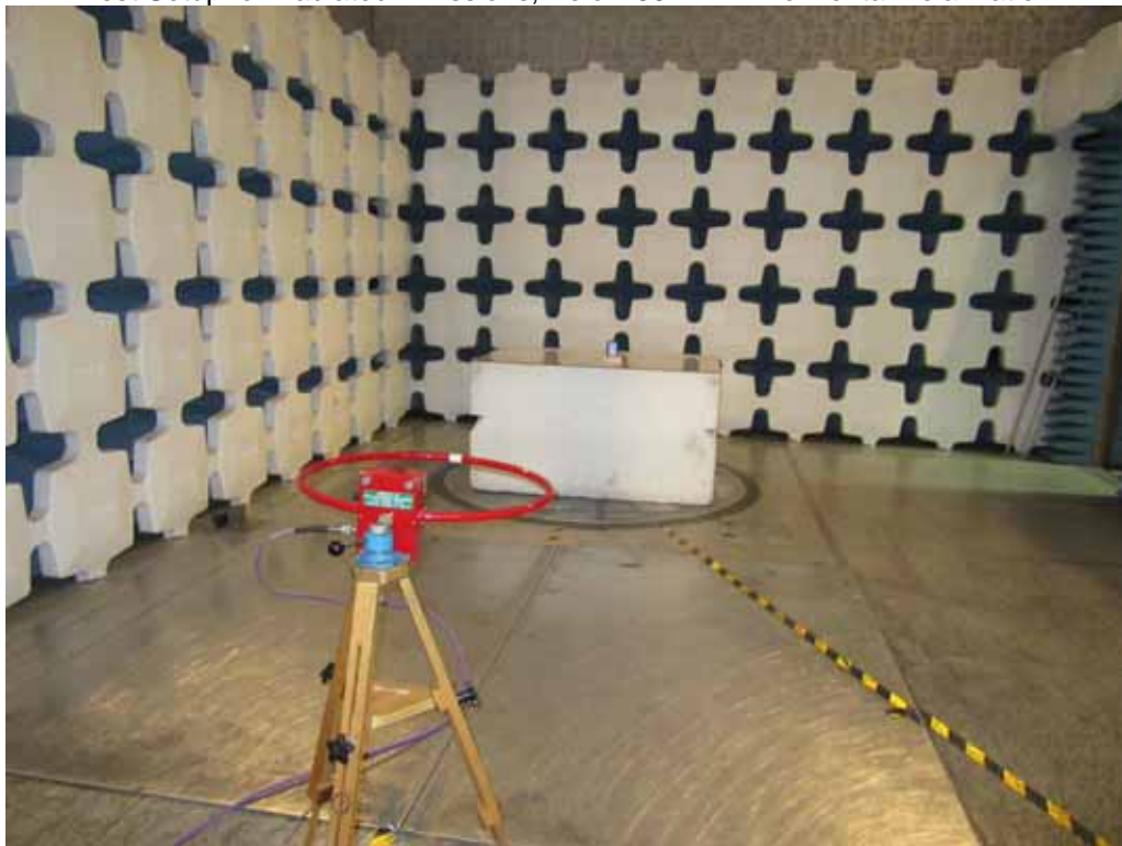
Test Setup for Radiated Emissions, Below 30MHz – Vertical Polarization
