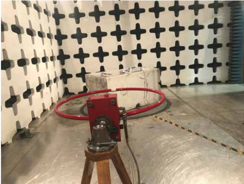
Test Setup for Radiated Emissions, 30MHz to 1GHz – Horizontal Polarization
