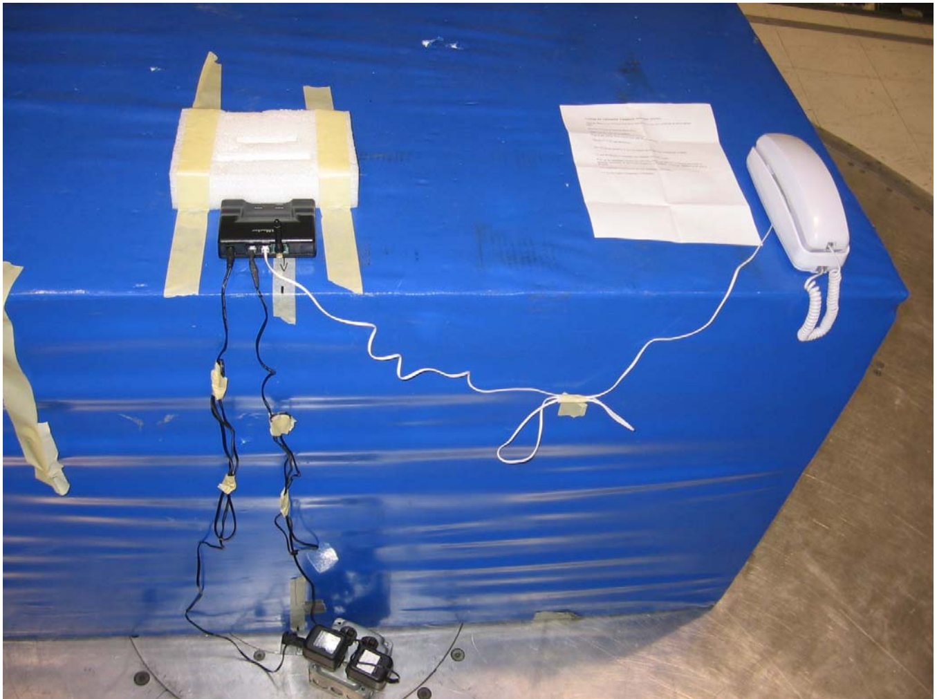
Figure 6 Test setup for Radiated Emissions
