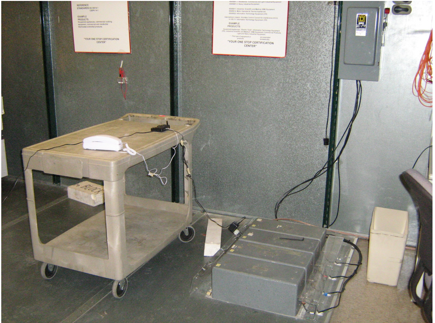
Figure 1 Test Setup for Conducted Emissions
