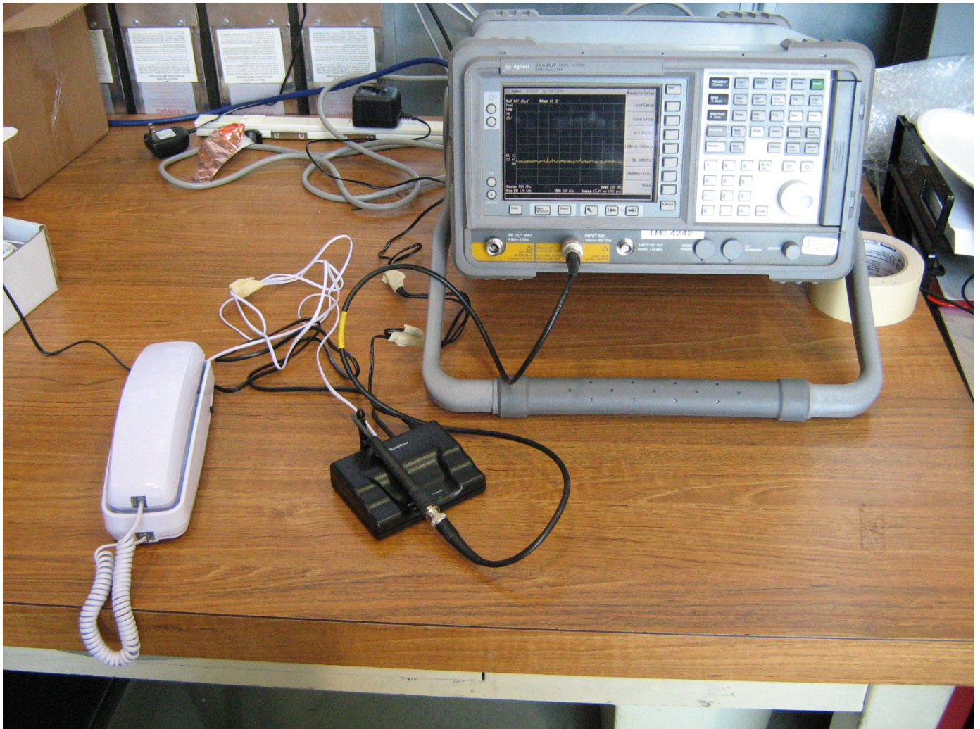
Figure 12 Test Setup for Occupied Bandwidth
