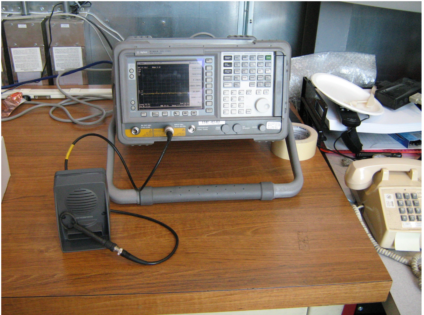
Figure 7 Test Setup for Occupied Bandwidth
