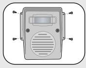
Mount PIR Motion Sensor vertically on solid surface a few feet off the ground and within 1000' of Base Station. Unit should be able to swivel as needed.
