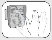
Test PIR Motion Sensor by waving hand in front of sensor. Test light should flash after several seconds.
