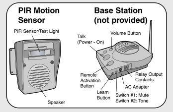
**On/Off:** To turn Base Station OFF hold down the Volume button until a beep is heard and light goes out. To turn Base Station ON press the Talk button.
