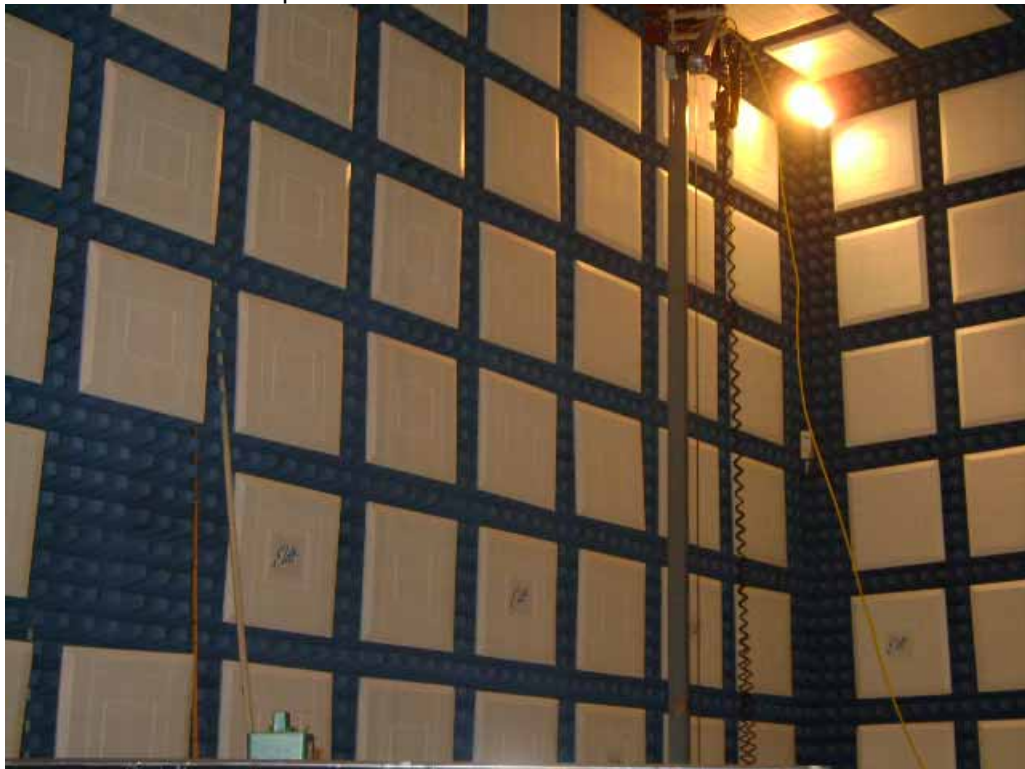
Test Set-up for Radiated Emissions – Vertical Polarization
