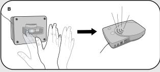
**B** Within 5 seconds, wave hand in front of PIR Motion Sensor. Test light will illuminate and Base Station will buzz.
