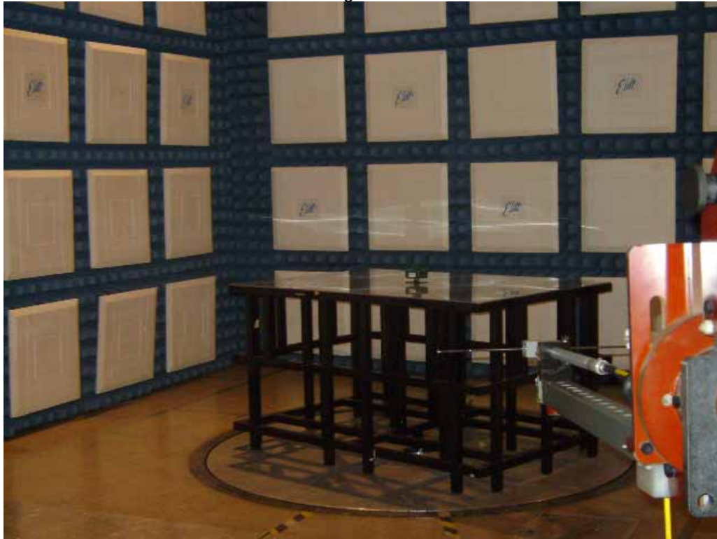
Test Set-up for Radiated Emissions – Horizontal Polarization
