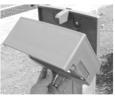
By placing the grooved bottom of the front panel under the front of the mounting plate and pushing the Gate Access Unit on to the mounting plate, then lock it into place using the included key. You will hear a periodic low-volume beep, indicating that the unit is operational and ready to be programmed with your secure master PIN number.
