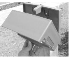
Clip the unit onto the already installed back plate, by placing the grooved bottom of the front panel under the mounting plate and push the Gate Access Panel up, on to the mounting plate, then lock it using the included key.
