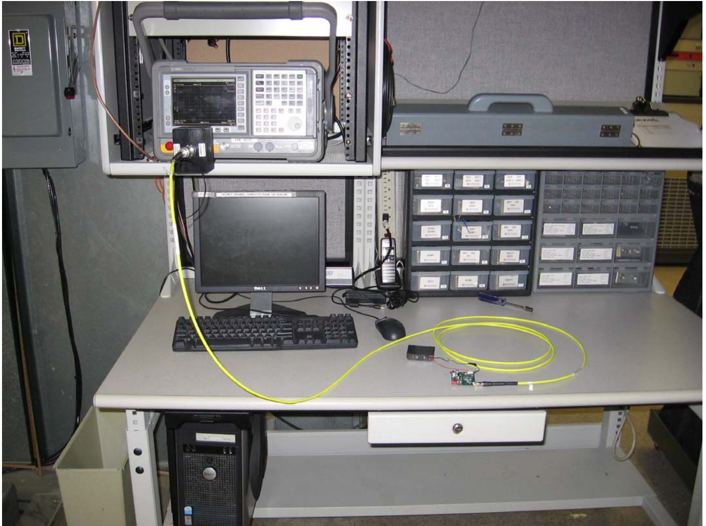
Figure 17 Antenna Conducted Measurements Test Setup
