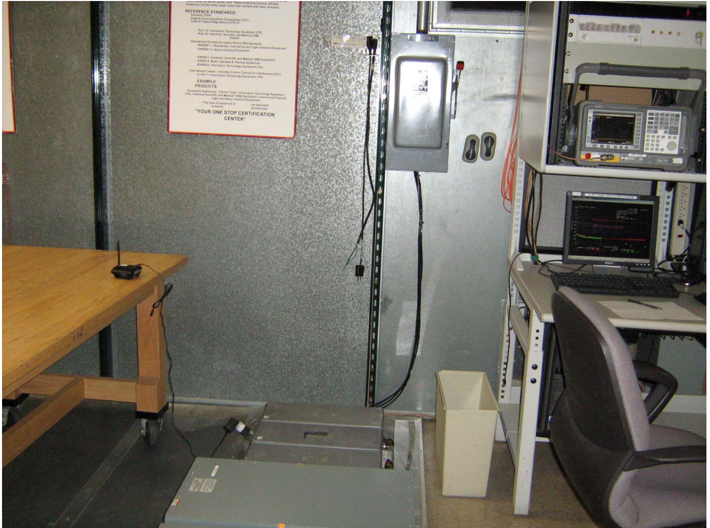
Figure 19 Line Conducted Emissions Test Setup
