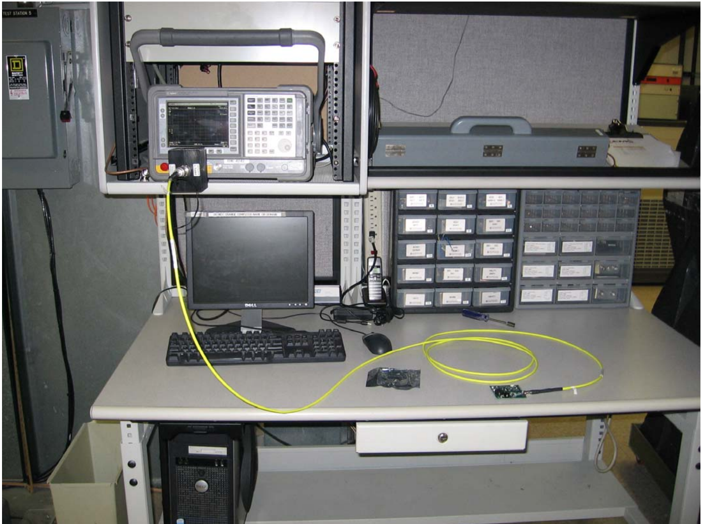
Figure 20 Antenna Conducted Measurements Test Setup
