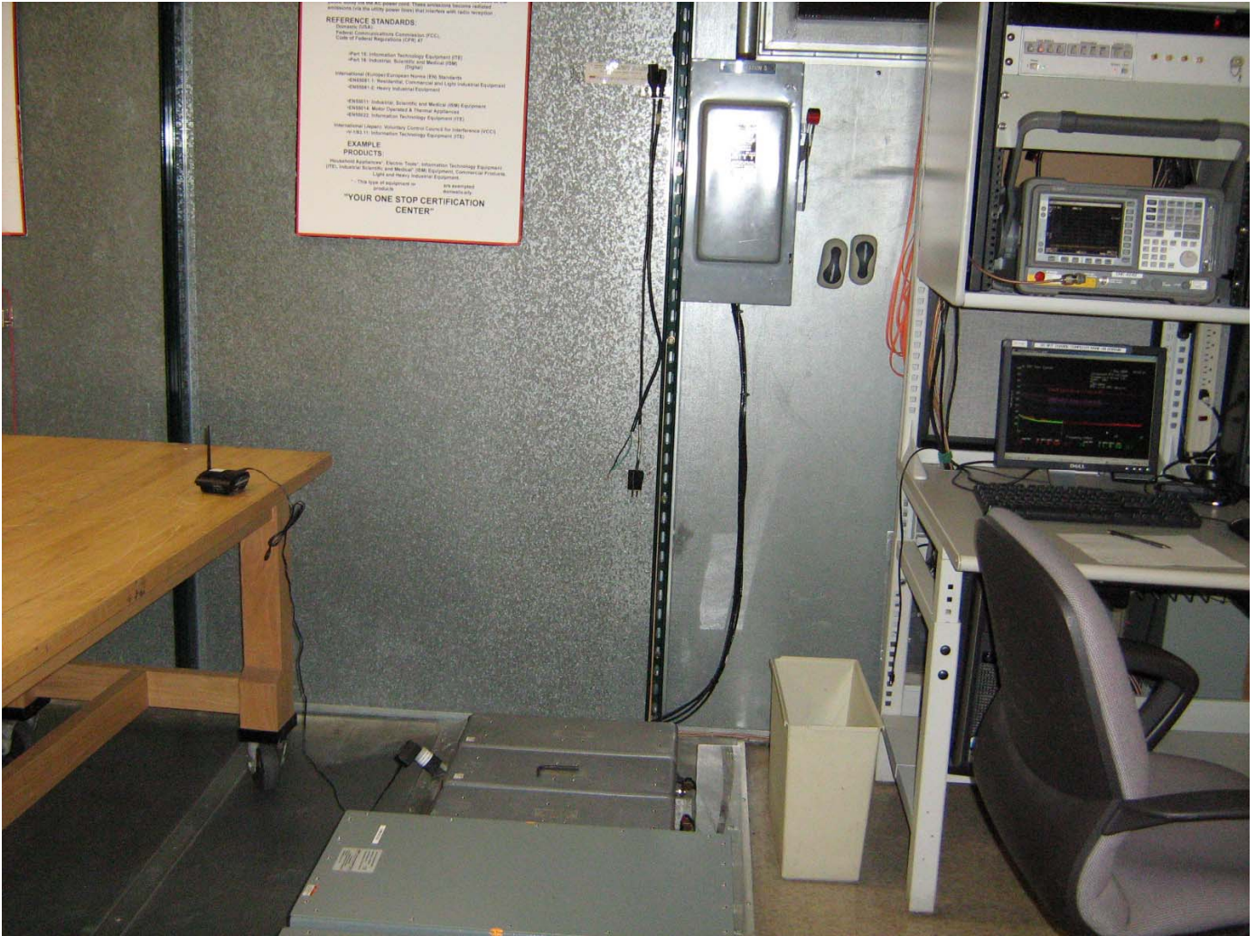
Figure 19 Line Conducted Emissions Test Setup
