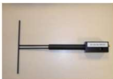
Figure 1 – Satimo COMOSAR Validation Dipole
