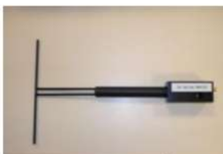
Figure 1 – Satimo COMOSAR Validation Dipole
