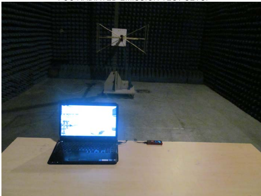
FCC RADIATED EMISSION TEST SETUP
