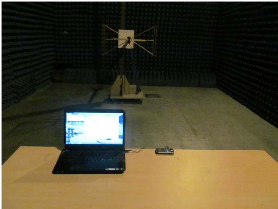
FCC RADIATED EMISSION TEST SETUP
