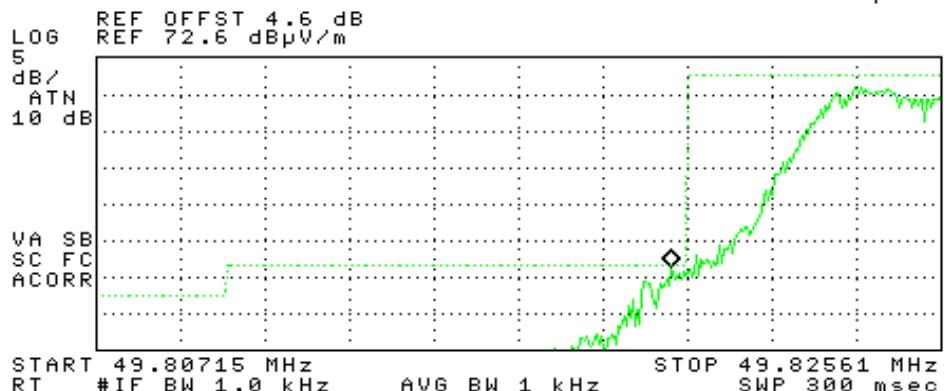
Alpha Unit - Low Channel. All out-of-band signals below the limit.
