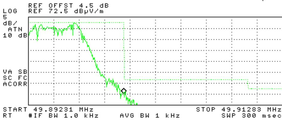
Alpha Unit - High Channel. All out-of-band signals below the limit.
