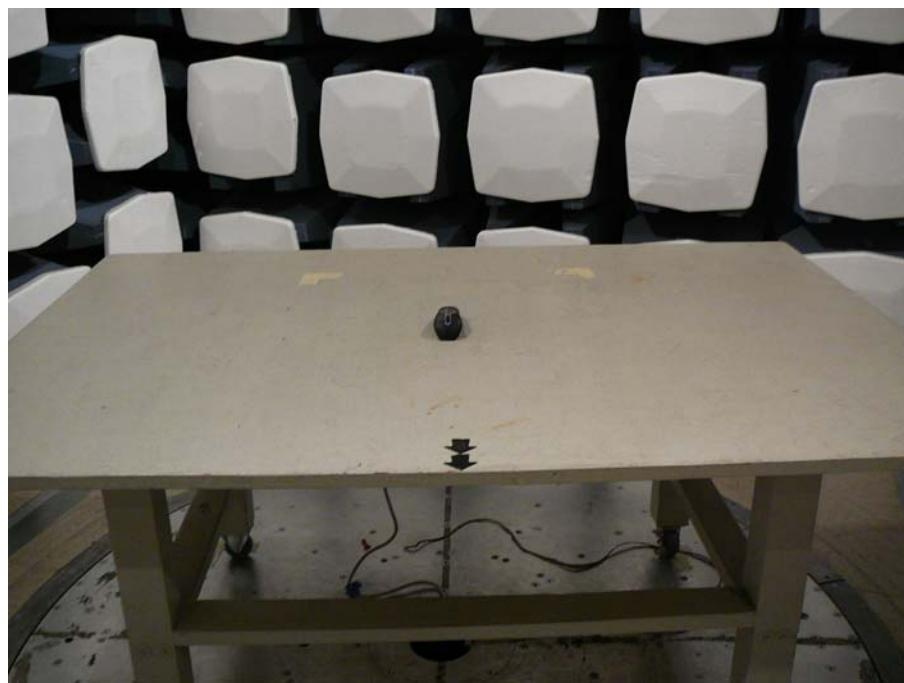
**15.4 Radiated Emission above 1 GHz Front View @ 3 Meters**
