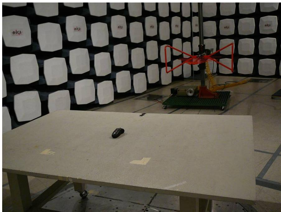
**15.3 Radiated Emission above 1 GHz Front View @ 3 Meters**
