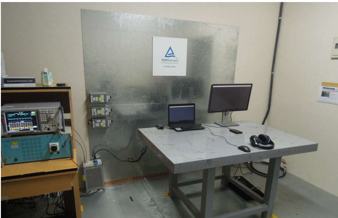
Photograph 5: Set-up for for Mains Conducted testing Front
