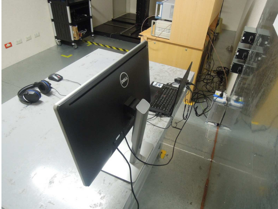
Photograph 4: Set-up for for Mains Conducted testing Back
