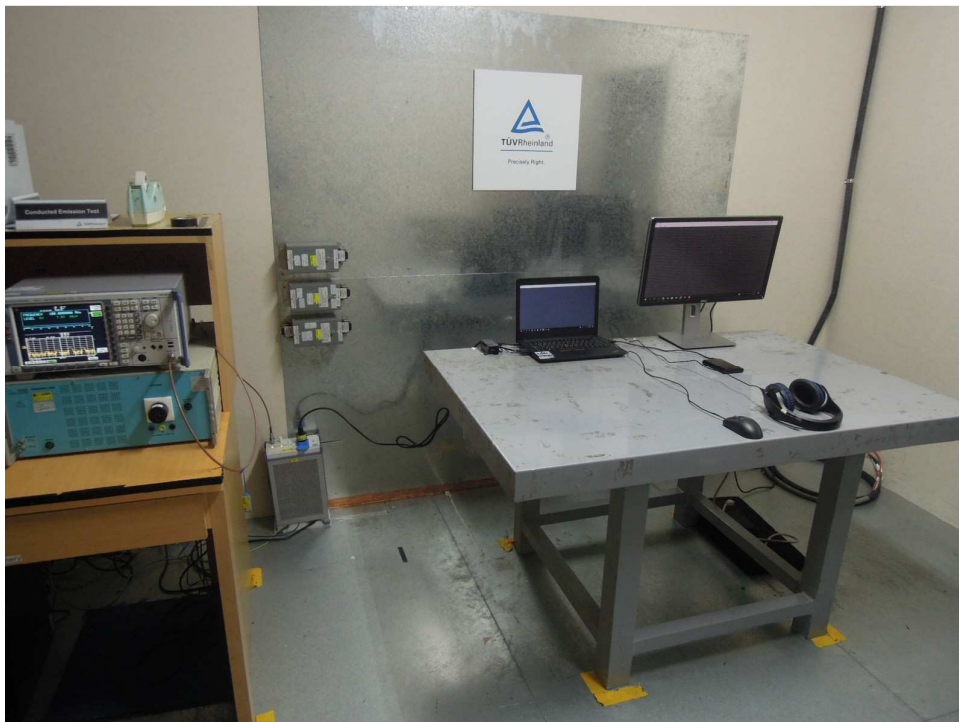
Photograph 5: Set-up for for Mains Conducted testing Front
