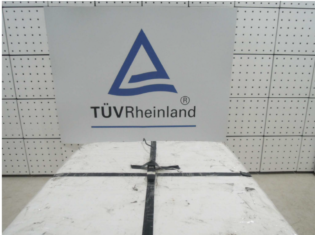
Photograph 6: Set-up for Spurious Emissions (Z axis orientation pre-test)
