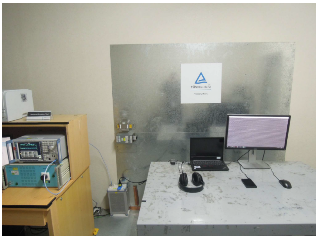
Photograph 9: Set-up for for Mains Conducted testing Front
