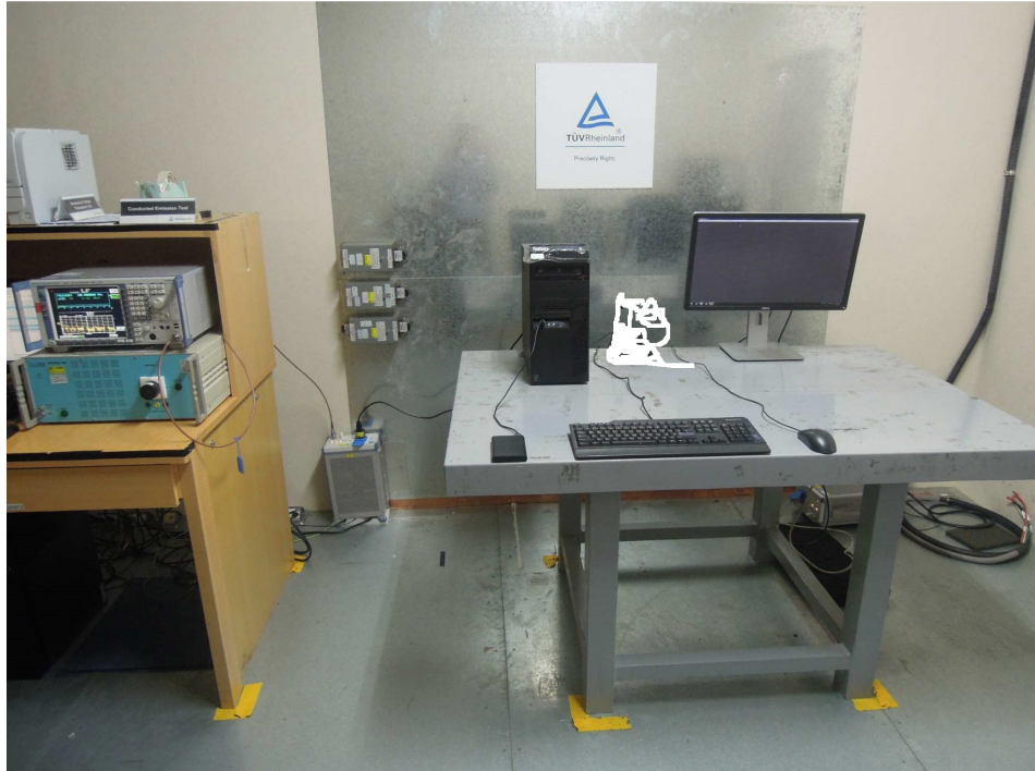
Photograph 6: Set-up for for Mains Conducted testing Front
