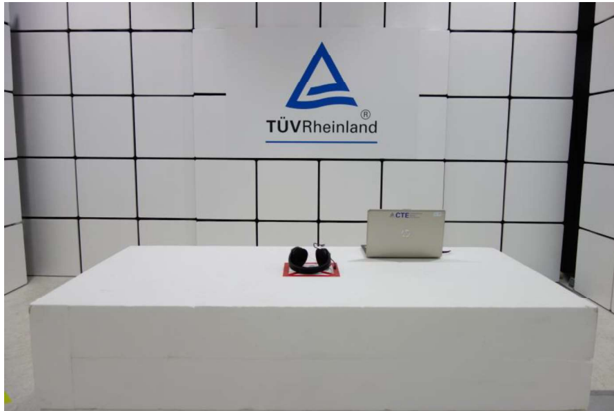
Photograph 1: Set-up for Spurious Emissions (Front View 1)
