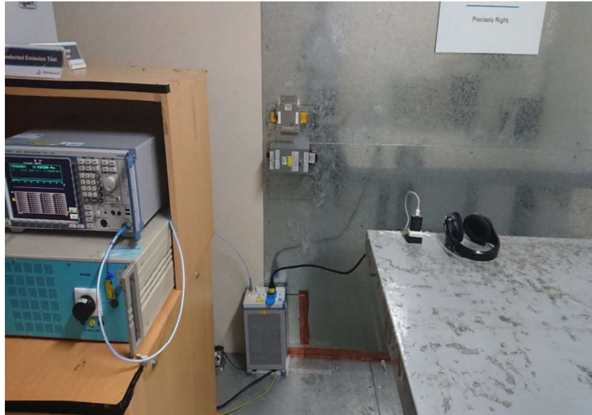
Photograph 9: Set-up for Mains Conducted testing Front
