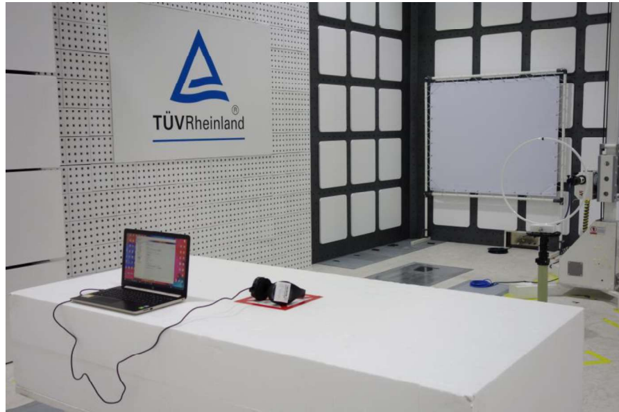
Photograph 3: Set-up for Spurious Emissions (Back View 1)
