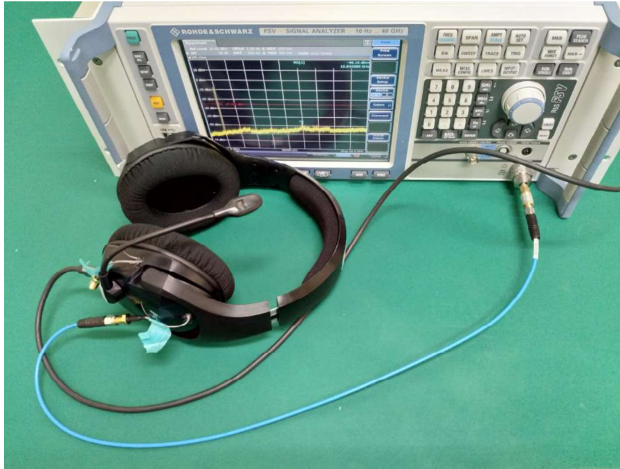
Photograph 7: Set-up for Conducted testing
