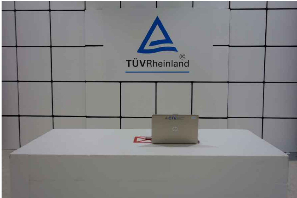
Photograph 1: Set-up for Spurious Emissions (Front View)
