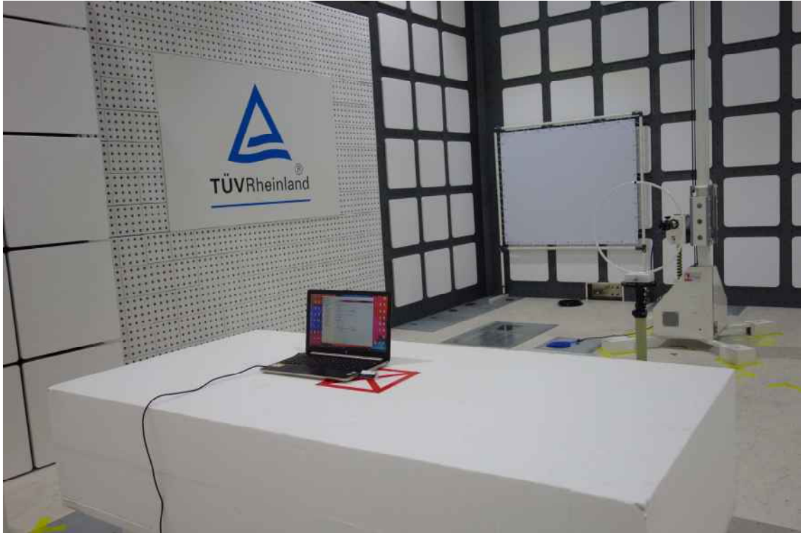
Photograph 2: Set-up for Spurious Emissions (Back View 1)
