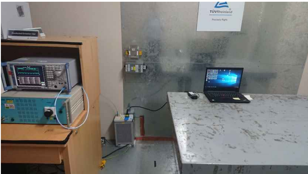
Photograph 5: Set-up for for Mains Conducted testing Front
