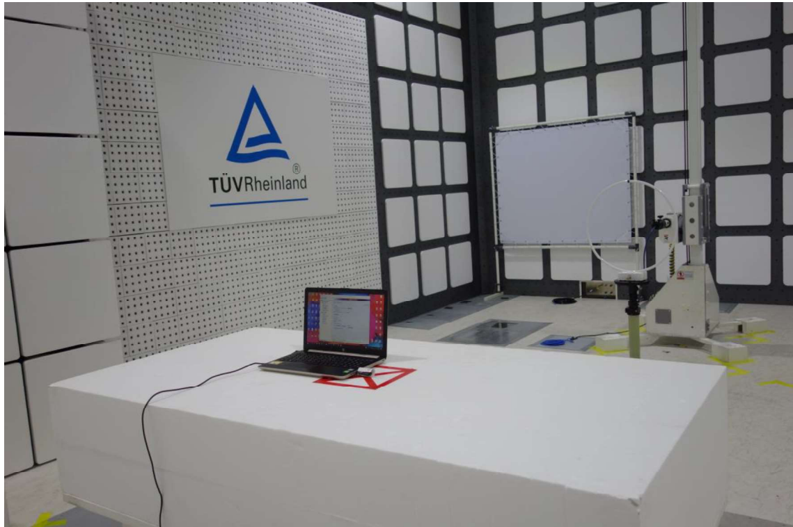
Photograph 2: Set-up for Spurious Emissions (Back View 1)
