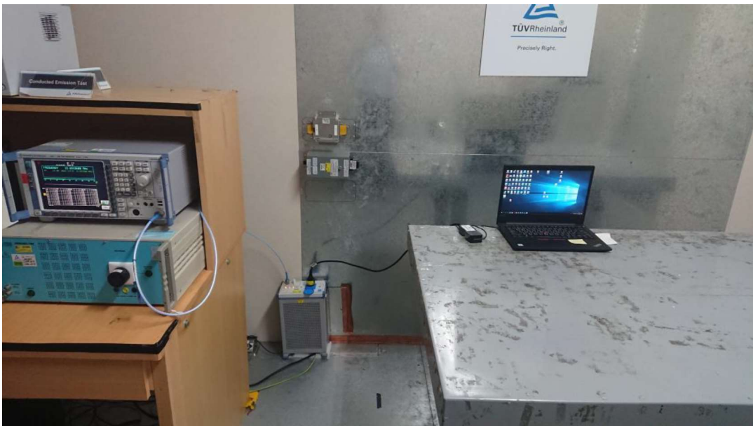
Photograph 5: Set-up for for Mains Conducted testing Front
