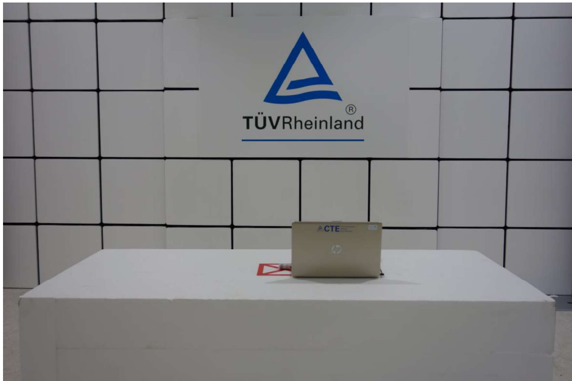
Photograph 1: Set-up for Spurious Emissions (Front View)
