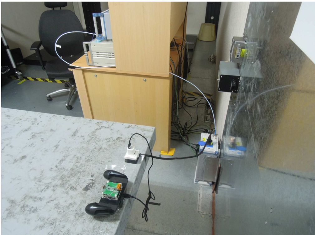
Photograph 4: Set-up for for Mains Conducted testing Back
