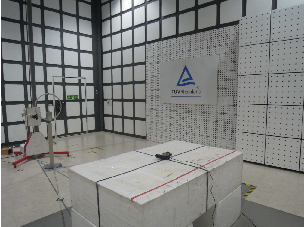
Photograph 3: Set-up for Spurious Emissions (Back View 2)
