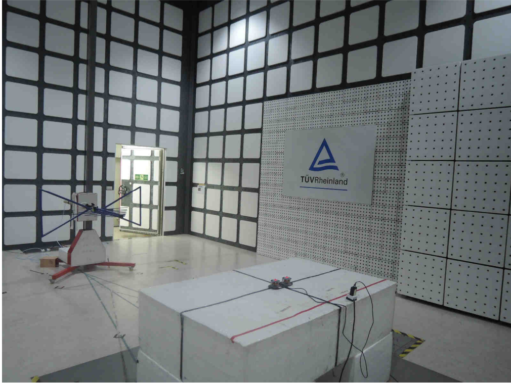
Photograph 3: Set-up for Spurious Emissions (Back View 2)
