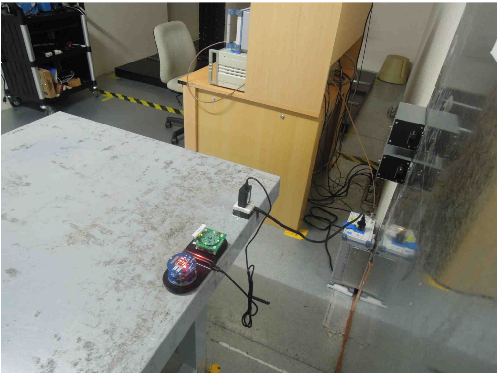
Photograph 4: Set-up for for Mains Conducted testing Back
