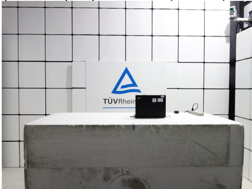
Photograph 2: Test Setup for Spurious Emissions (Front View 2)
