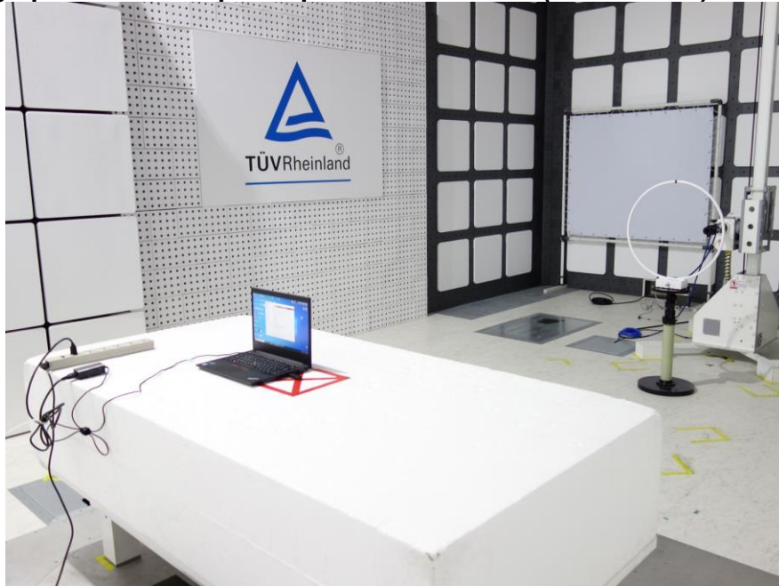
Photograph 6: Test Setup for Spurious Emissions (Back View 4)
