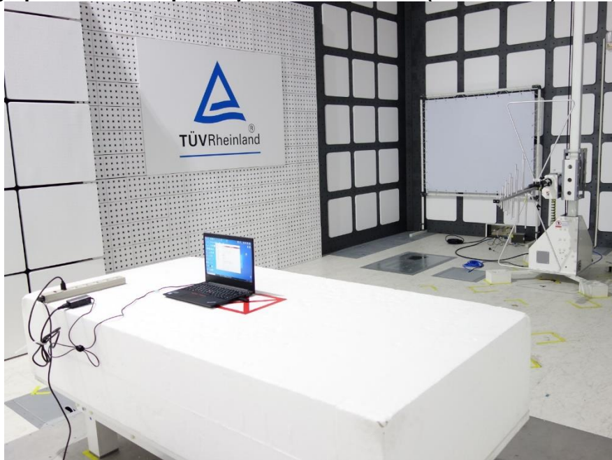
Photograph 4: Test Setup for Spurious Emissions (Back View 2)
