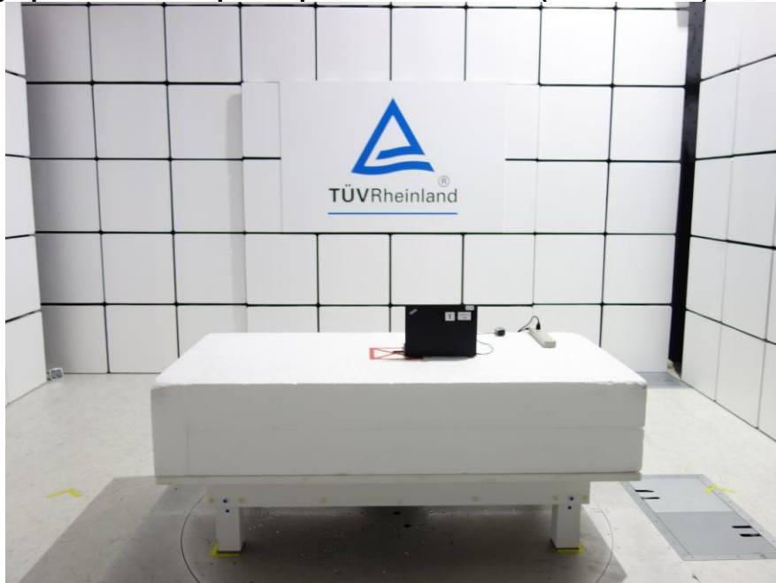
Photograph 2: Test Setup for Spurious Emissions (Front View 2)
