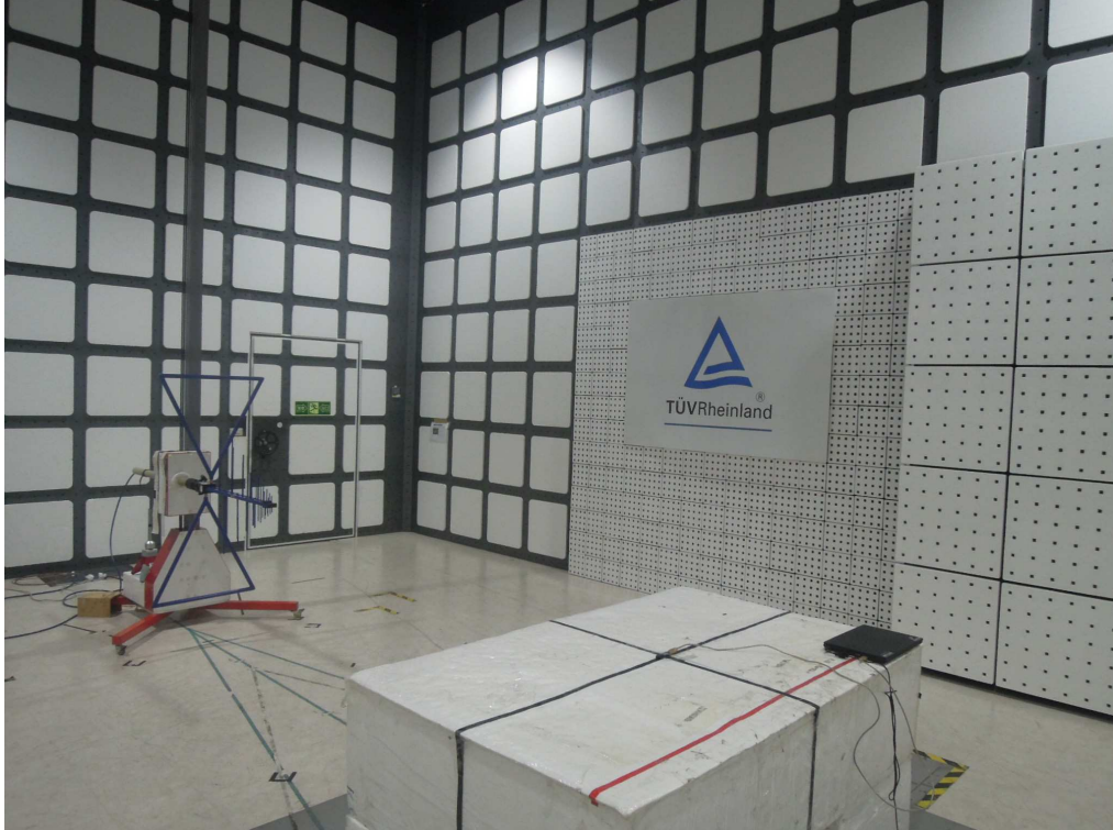
Photograph 2: Set-up for Spurious Emissions (Back View 1)
