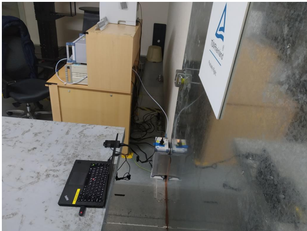
Photograph 7: Set-up for AC Mains Conducted Testing (Back View)
