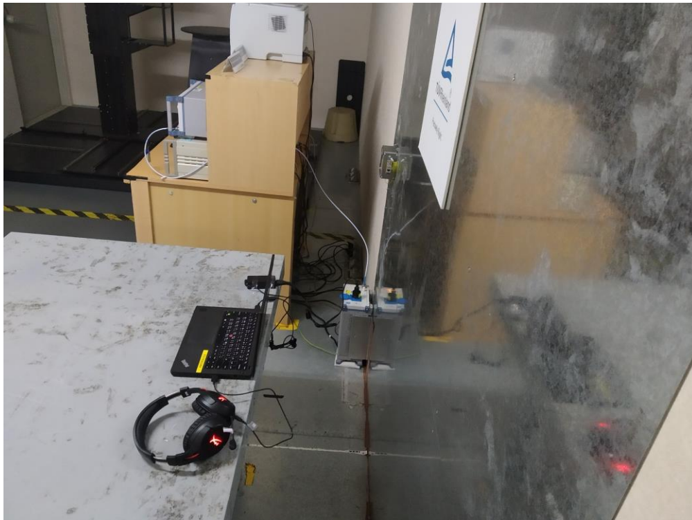
Photograph 8: Set-up for Mains Conducted Testing (Back View)
