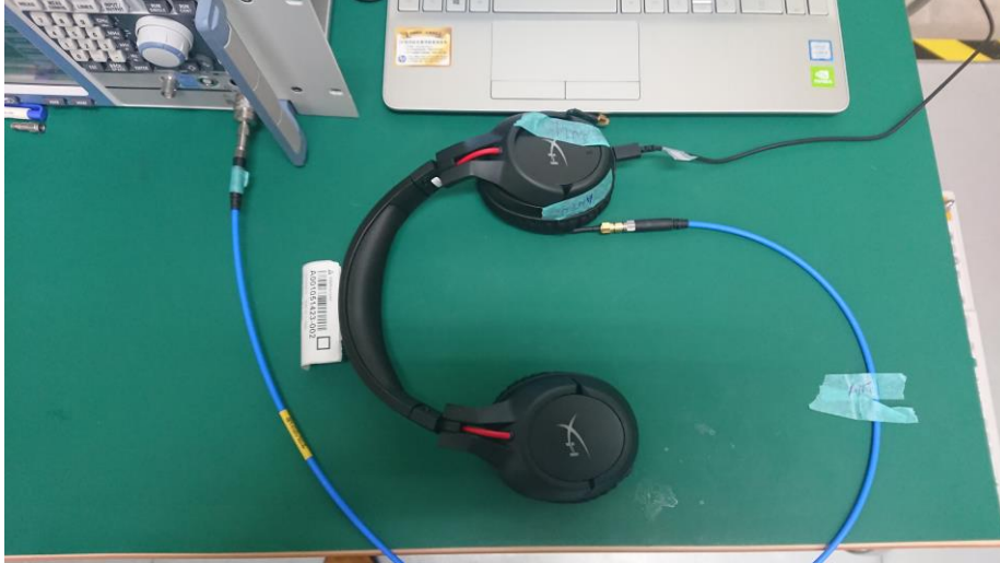
Photograph 7: Set-up for Conducted Testing
