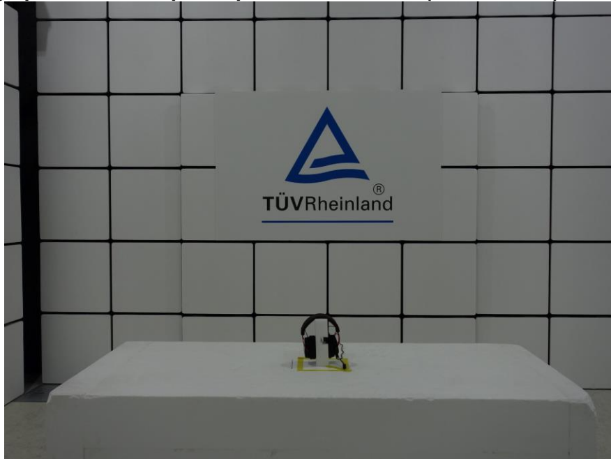
Photograph 1: Test Setup for Spurious Emissions (Front View 1)
