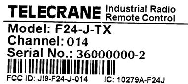
Labels are printed by thermal transfer on polyester stock with permanent adhesive, size 51 x 25 mm.
