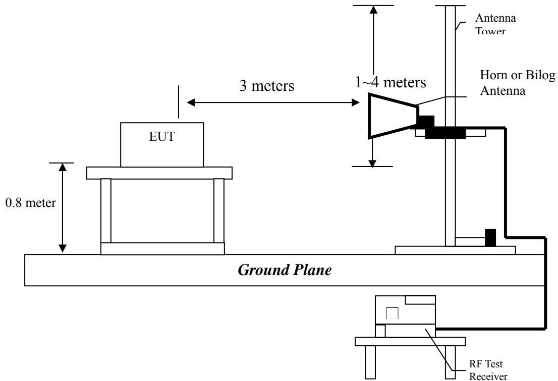
The signal is maximized through rotation and placement in the three orthogonal axes. Radiated emission measurements were performed from 30 MHz to 3.2 GHz. Spectrum Analyzer Resolution Bandwidth is 100 kHz or greater for frequencies 30 MHz to 1 GHz, 1MHz – for frequencies above 1 GHz.
