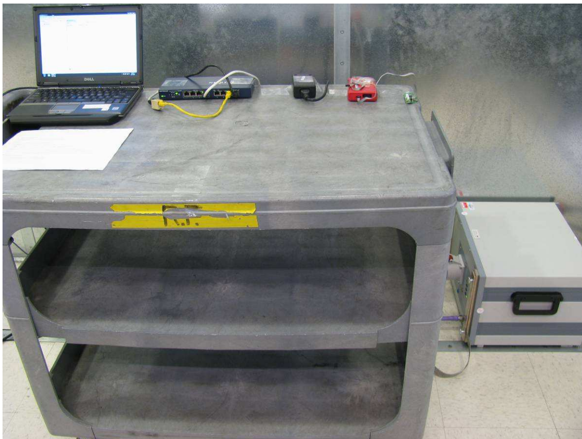
Conducted Power Port Emissions (Front)
