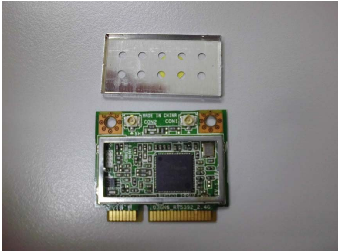
Figure 2 Removed Shielded Cover, Front View
