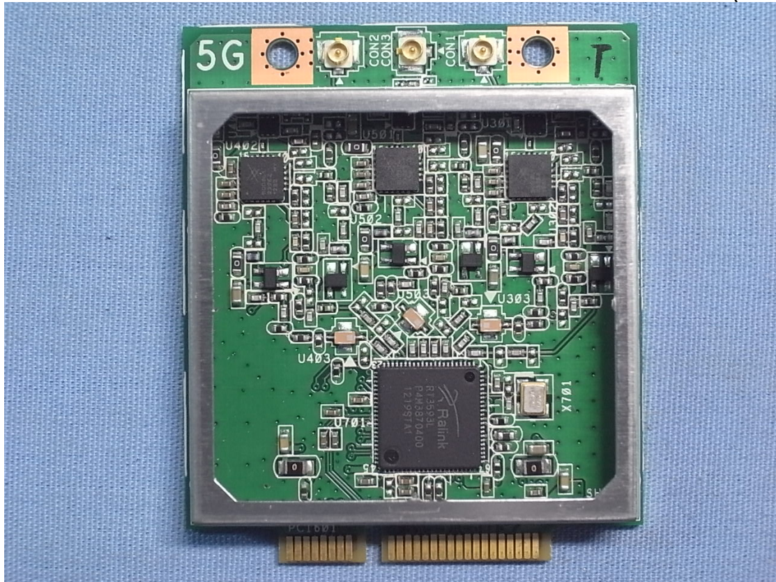
5GHz 802.11n 3T3R wifi module (Front View)
