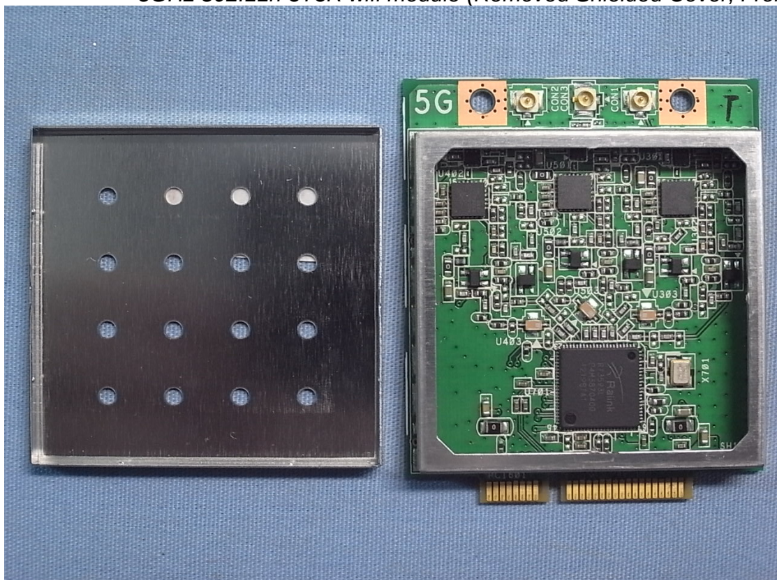
5GHz 802.11n 3T3R wifi module (Removed Shielded Cover, Front View)
