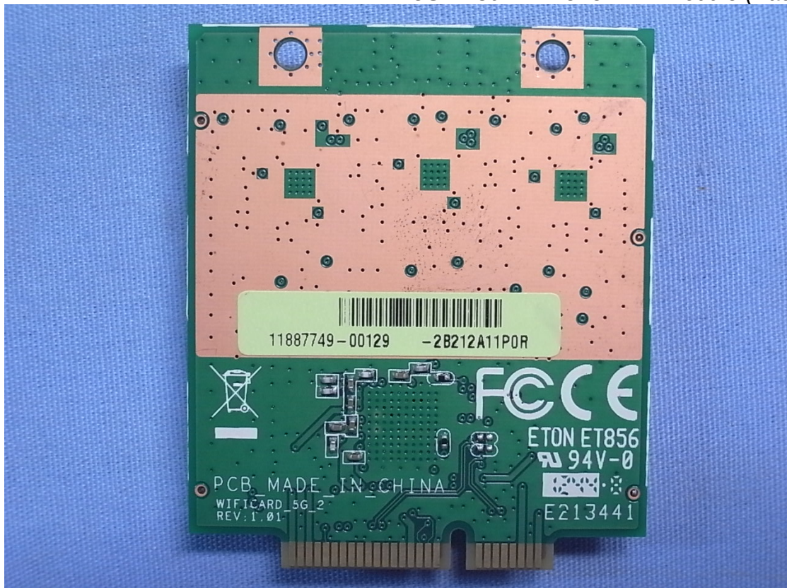
5GHz 802.11n 3T3R wifi module (Back View)
