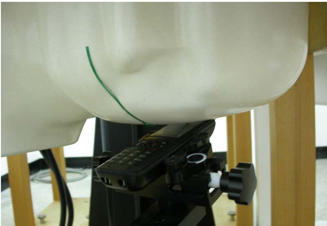
Measurement Position of Left-Tilt (LT) with Handset
