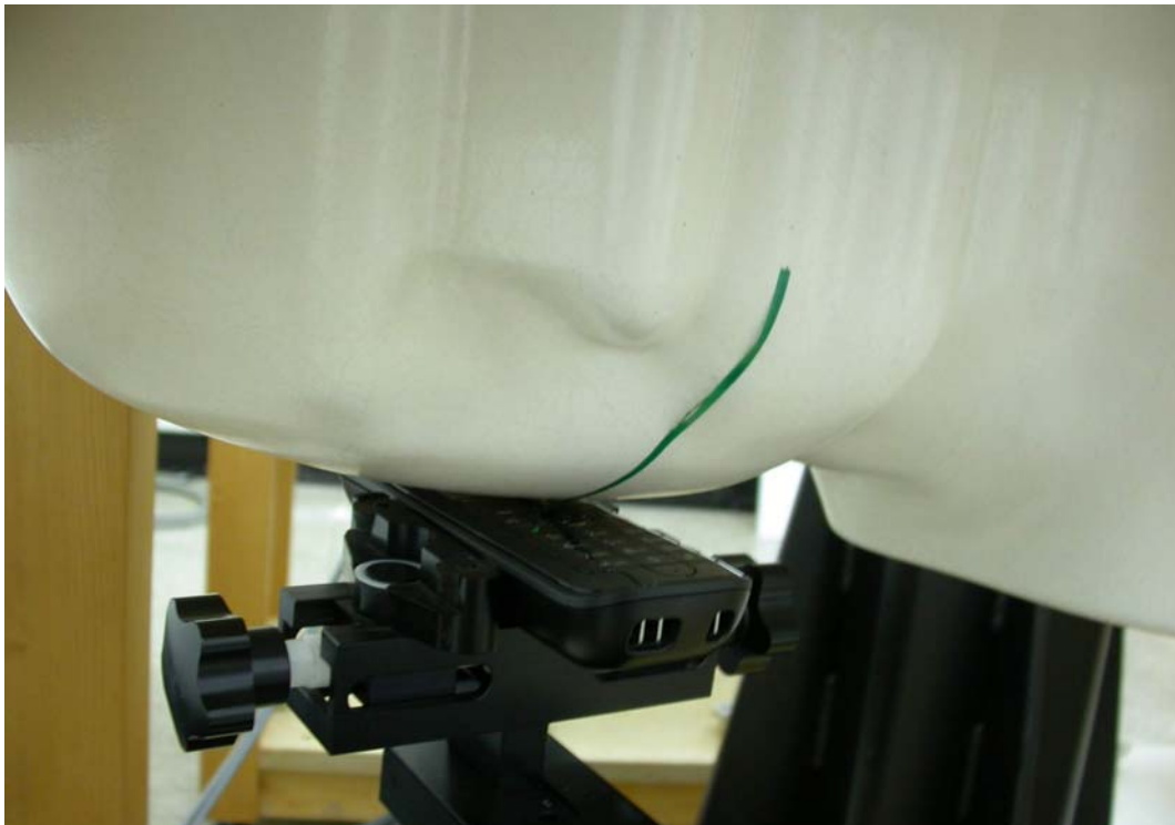
Measurement Position of Right-Cheek (RC) with Handset
