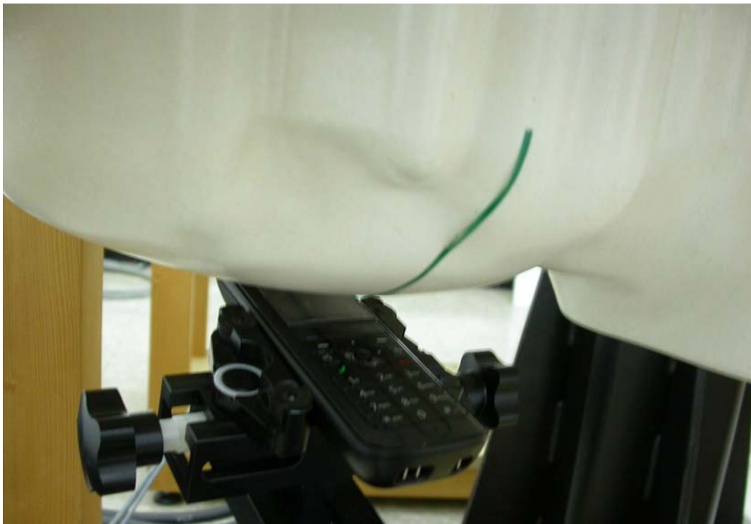
Measurement Position of Right-Tilt (RT) with Handset
