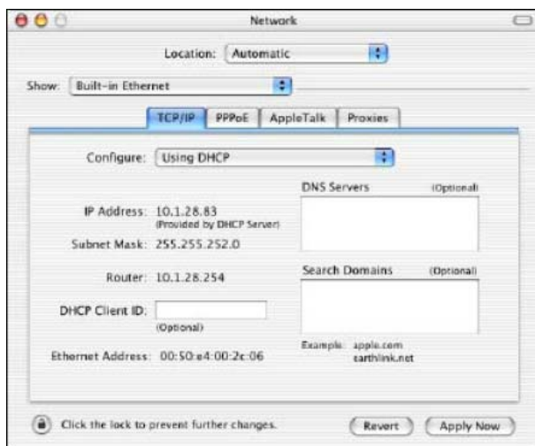
Figure 10. Selecting Using DHCP in the Configure Field
