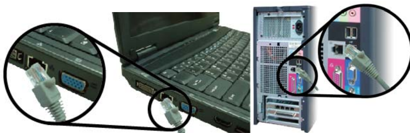
Figure 4. Connecting the Gateway to the a Laptop or Desktop Computer
