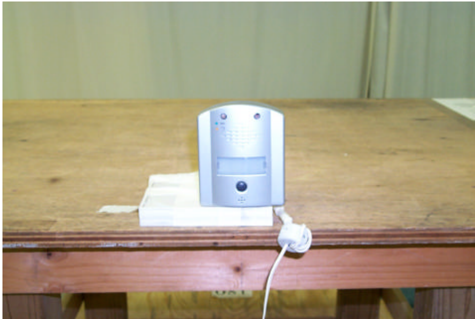
Figure 3.1 Radiated Test Setup, Position X-TX w/AC
