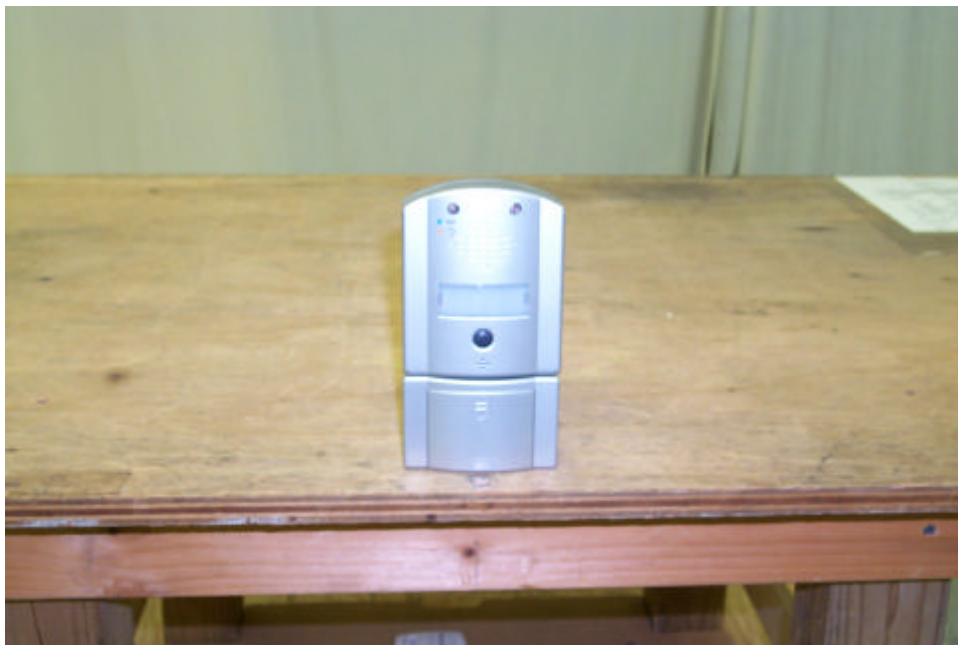
Figure 3.2 Radiated Test Setup, Position Y-TX w/ Battery Box
