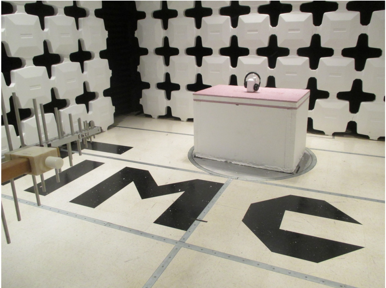
RADIATED EMISSIONS TEST SET UP PHOTO
