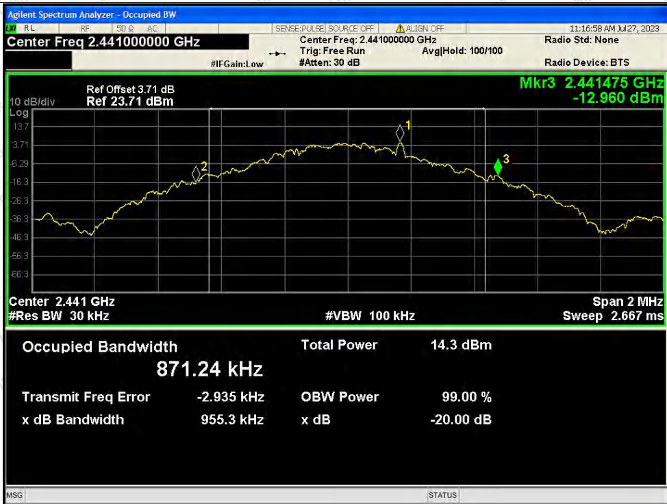
-20dB Bandwidth NVNT 1-DH5 2441MHz Ant1
