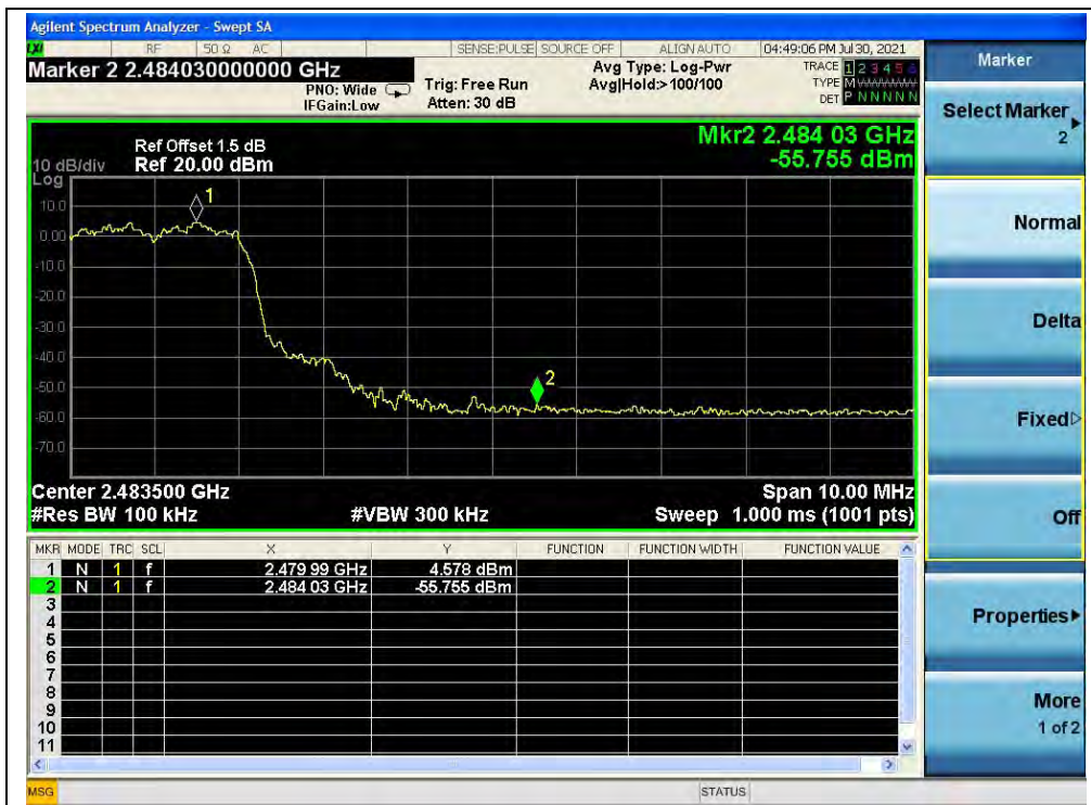
(Band edge with hopping on, Channel 78, 8-DPSK)
