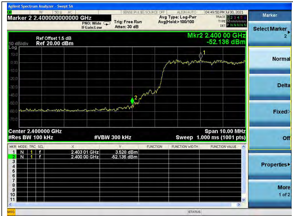
(Band edge with hopping on, Channel 0, 8-DPSK)
