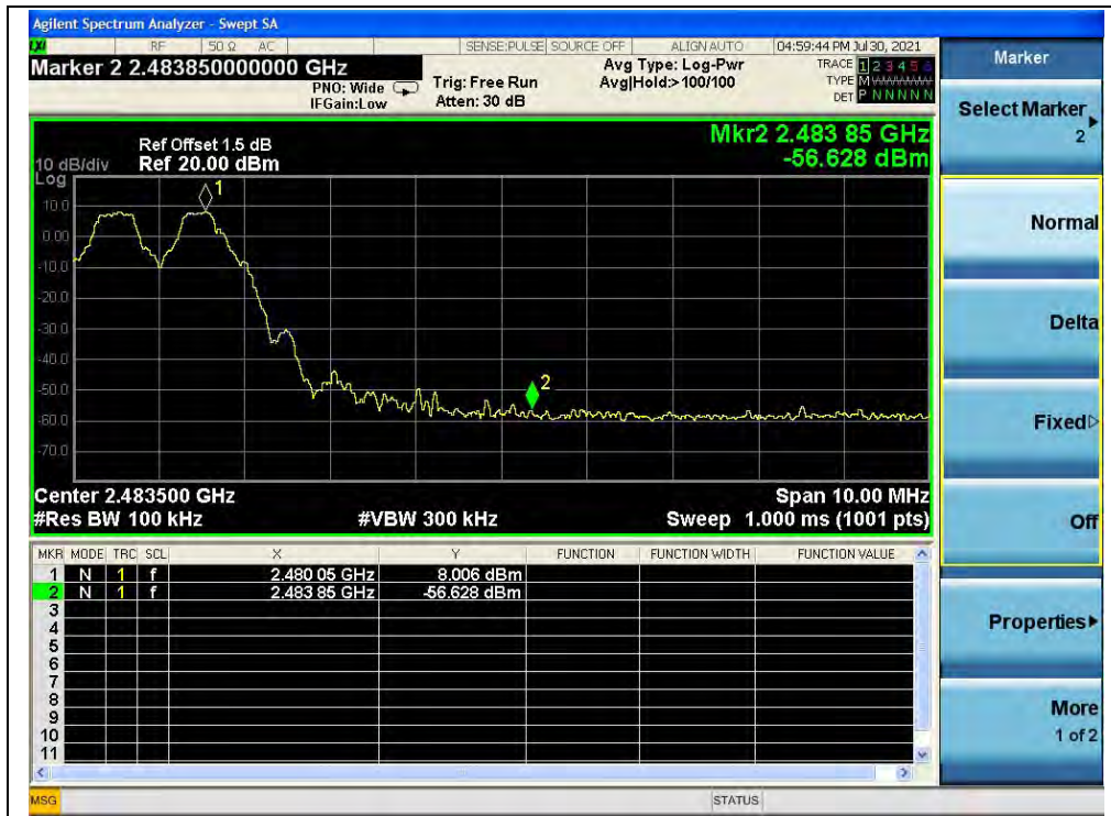
(Band edge with hopping on, Channel 78, GFSK)
