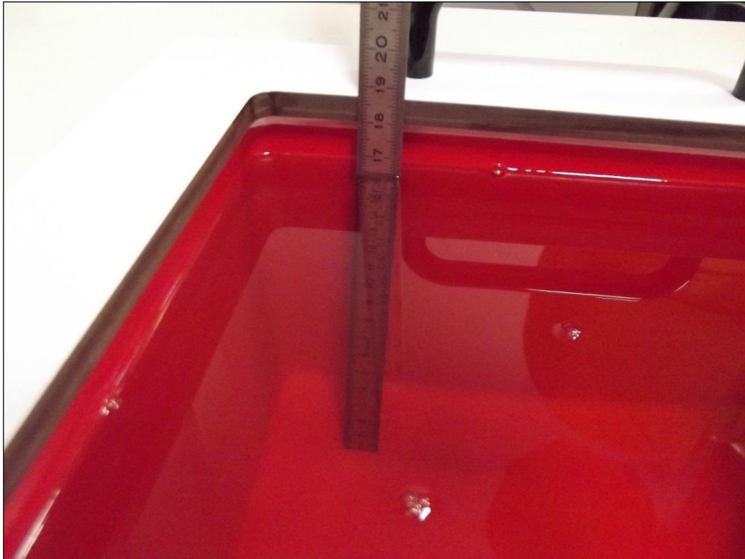
Photo 1: Liquid depth 450 MHz body simulating liquid
